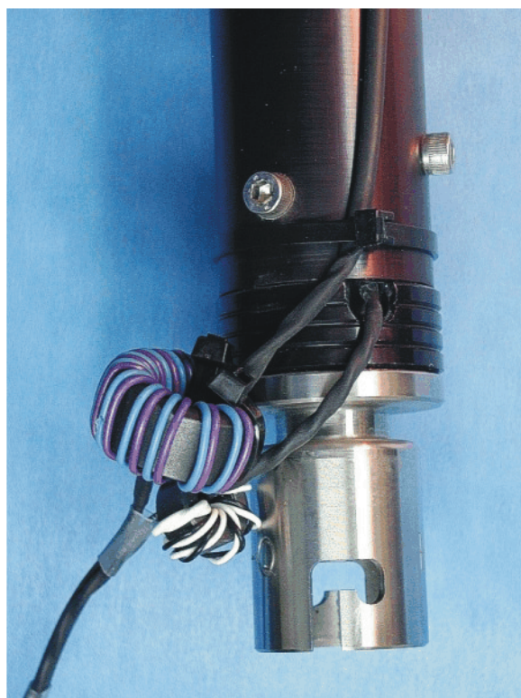
Ferrites used for RFI filtering at base
