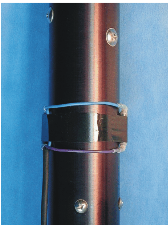
Reed Switches #1 & #2 - 180° apart
